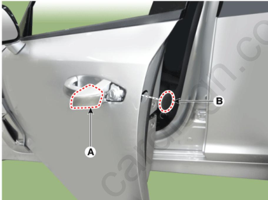
2. Remove the front door lock (A) after loosening the mounting bolt.
